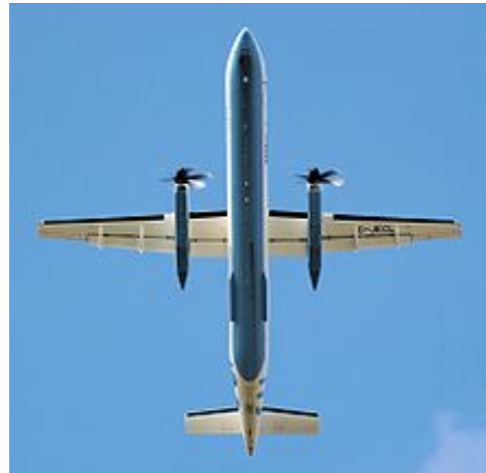
High aspect ratio wing ( AR=12.8 ) of the Bombardier Dash 8 Q400
