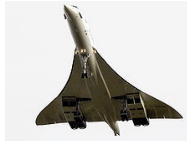
Very low aspect ratio wing ( AR=1.8 ) of the Concorde
