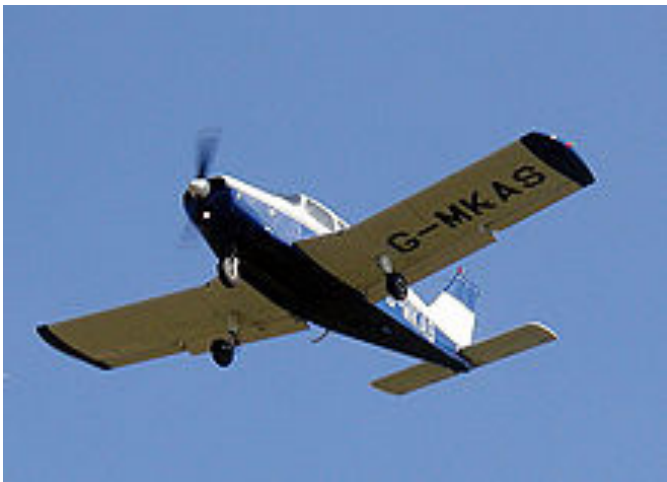
Low aspect ratio wing ( AR=5.6 ) of a Piper PA-28 Cherokee
