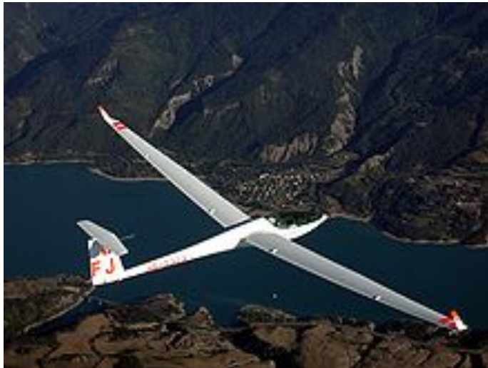
Very high aspect ratio wing of the Glaser-Dirks DG-808 glider ( AR=27.4 )
